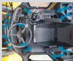
Air conditioning & heater
