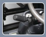
**Easy and safe shift lever** A single lever on the left side of the steering column gives the operator fast and easy controls of the direction.
