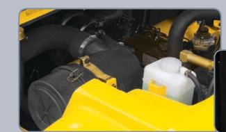
**Easy change air cleaner** The air filter is readily accessible for cleaning or replacement.
