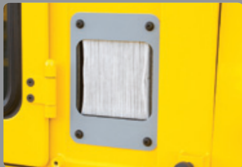
Cabin air fresh filter The internal pressure is maintained to be slightly higher than that of outside to exclude dust and to reduce noise levels.
